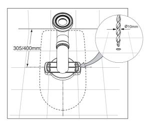
Using Ø10mm masonry drill bit, drill the floor to connect the floor fixing set, follow floor fixing set, follow in the figures.
