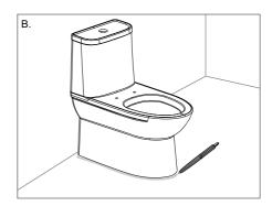
B. Set proprely the VC on the floor, mark the location to be drilled. (the figure just as reference)
