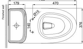
Dimensioning diagrams are provided for each model. Note: dimensions are nominal and may vary within the range of manufacturing tolerances.
