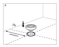
A. Insert the flange into the waste outlet pipe, ensuring that the arrow is pointing toward the floor.
