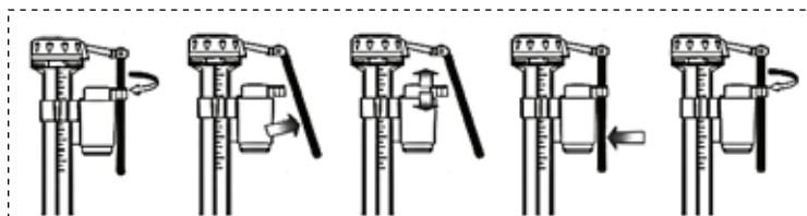
If water level in tank is below or higher than prescribed level a little bit adjust
