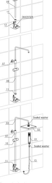
· Check up every step to ensure the stability and tightness to avoid any leaking before testing the shower spray.
