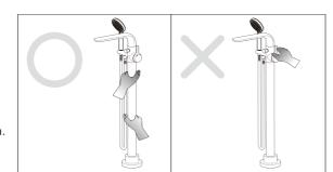
\* Warning: Avoid lifting/ holding product lever only during installation. Instead, hold product spout/ main body.
