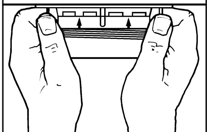
从水槽下面装上纤维垫圈和螺口支撑环到水槽凸缘，并按箭头指向
