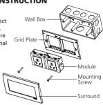
Insert a screwdriver into the clip lock, and twist the screwdriver to remove the surround.
