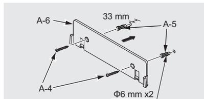
When mounting on a plaster board or tiled wall.
