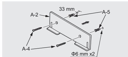
When mounting on a plaster board or tiled wall.
