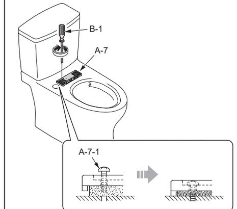
Failure to tighten screw A-7-1 completely will cause moving sideways of C-1.
